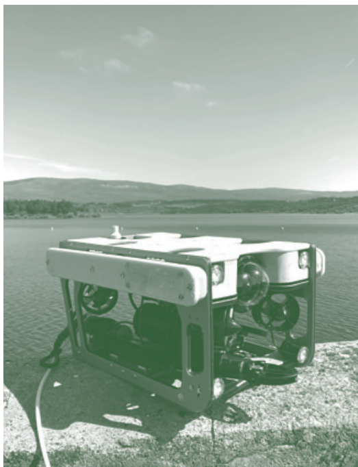
ROV used in the reservoir sampling campaign of the SOS-AGUA-XXI project.
