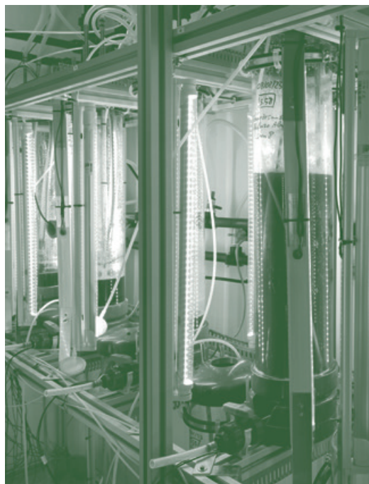
Experimental plant for microalgae cultivation for nutrient removal.
